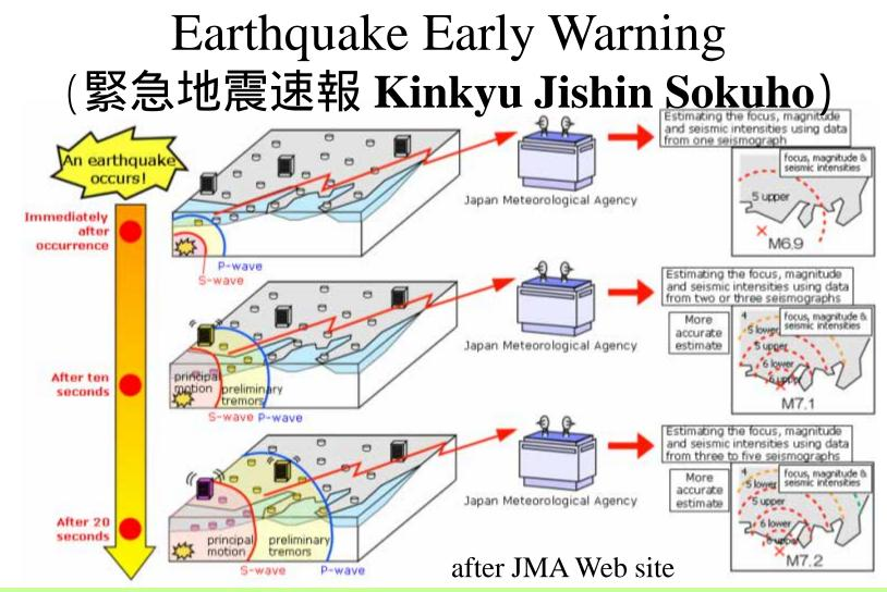
The EEW system provides advance warning of estimated seismic intensities and expected arrival time of S-waves. These estimates are based on prompt analysis of hypocenter location and earthquake magnitude using data observed by seismographs near the epicenter. The system issues several EEW messages during the course of one earthquake, improving the accuracy of the warning as the amount of available data increases.
