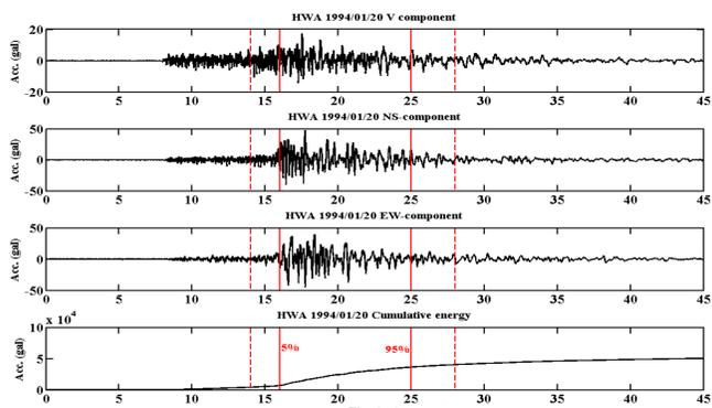
Figure 1 An example of the duration time of strong ground motion record by the acceleration seismogram of HWA station. The red dash lines show the time interval between the first and the last amplitude which equal to or greater than 10gal. The red lines show the interval across the dissipated energy within 5%~95% of the total energy of the interval of dash lines.
