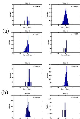
Figure 13 Histogram of the residual of the logarithm duration for site classes B, C, D, and E. The  $\sigma$  are standard deviation values. (a) for the earthquakes within  $M_L=5.0-7.0$  from 2011 to 2012 (b) for Chi-Chi earthquake
