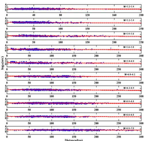
Figure 4 Logarithm of strong shaking duration time decay with distance for 0.2 magnitude interval of  $M=5.0-7.0$ . The red lines show the best regression of the data and red dash lines show the  $\pm$ RMS range (68% of data in this range).
