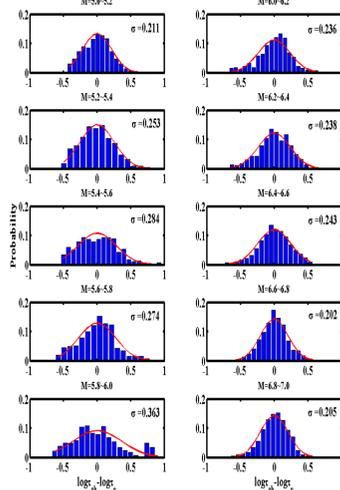
Figure 5 The probability density of the residuals of Logarithm duration time for 0.2 magnitude interval of  $M=5.0-7.0$ . The reds display the normally distribution.
