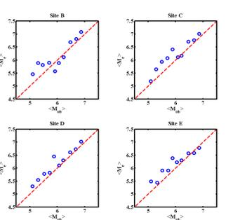
Figure 10 The comparison of the average of the estimated magnitude  $\langle M_e \rangle$  to the observed magnitudes  $\langle M_{ob} \rangle$  for magnitude in 0.2 interval for site classes B, C, D, and E.
