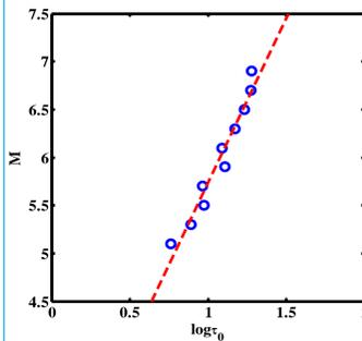
Figure 6 The regressed relationship between the strong shaking duration at 0 km distance ( $\tau_0$ ) and magnitude (M).
