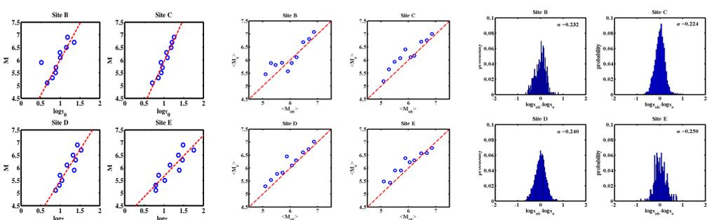
Figure 9 The regression of relationship of strong shaking duration at zero distance ( $\tau_0$ ) and magnitude (M) for different site classes.
