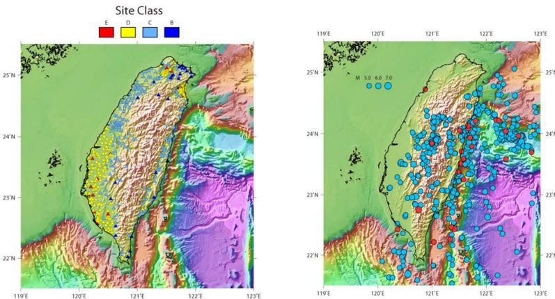
Figure 2 Distribution of strong-motion stations of Taiwan Strong Motion Instrumentation Program (TSMIP). The colors denote the site classifications as defined by Kuo et al. (2012).
