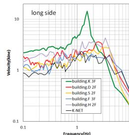
Fig.9 Velocity response spectrum calculated with waveforms recorded by "i-jishin" terminals
