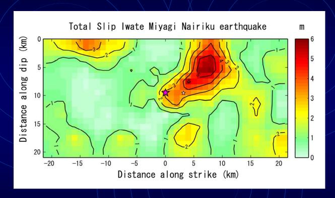
Maximum slip 5.7m average rupture velocity 1.8 km/s
