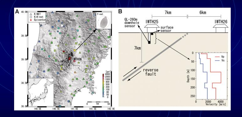
Borehole accelerometer is located at –GL/260m at an S-wave velocity layer of 1800 m/s
