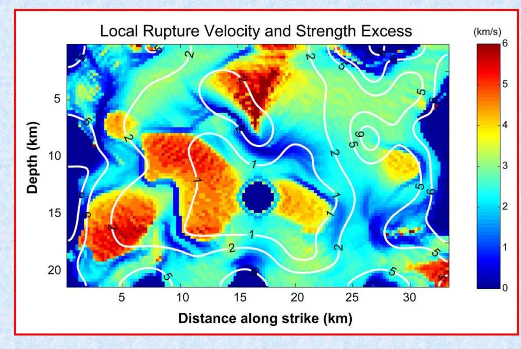
White lines denote the strength excess from dynamic model (in MPa).
