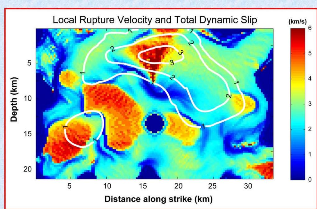
These panels show the calculation of the local rupture velocity obtained as the inverse of the gradient of rupture times from the dynamic model. They reveal a large heterogeneity of the rupture velocity across the fault plane.
