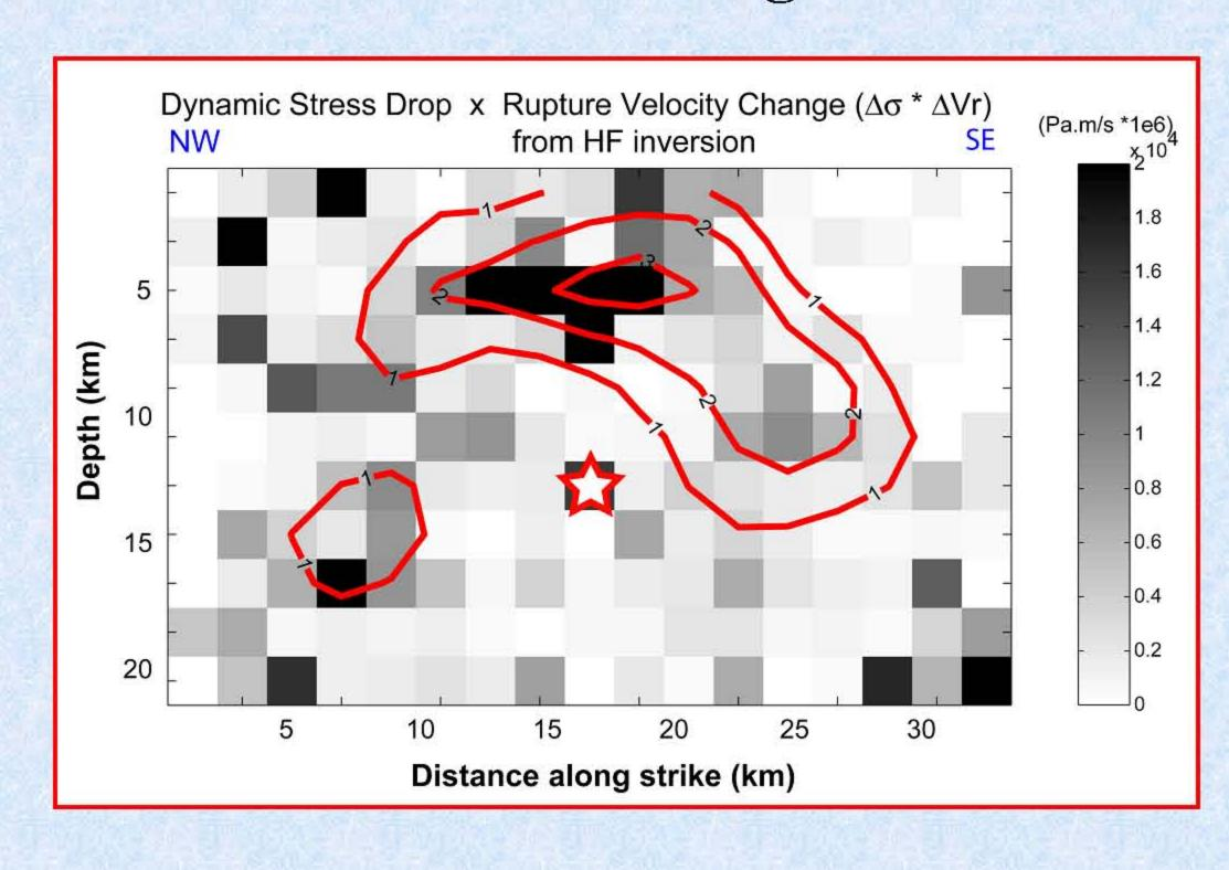
This picture shows a preliminary result of the HF radiation from the source obtained by inversion of HF near-fault ground motion (gray shading). The red lines correspond to the total slip from dynamic model.
