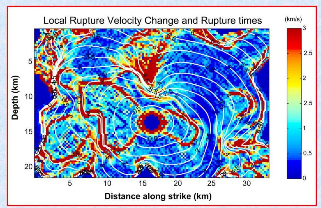
This picture shows the change in rupture velocity across the fault plane. We can observe that the largest slip region in the fault plane has a very strong rupture velocity gradient.
